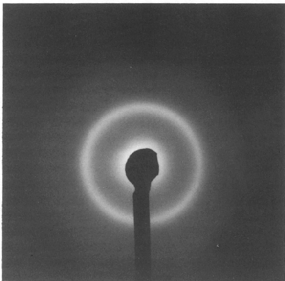
Figure 3 An electron diffraction pattern (TEM, 100 kV) from the near-surface region of \{10\bar{1}2\} sapphire implanted with 5 \times 10^{17} Y ions/cm 2 . The pattern shows diffuse rings characteristic of an amorphous material.
